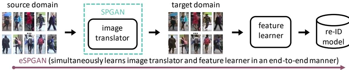
Fig. 1. Pipeline of the “learning via translation” framework. First, we translate the labeled images from a source domain to a target domain. Second, we train re-ID models with the translated images using supervised feature learning methods. SPGAN is only used to improve the first component of the framework, while eSPGAN simultaneously learns the two components in an end-to-end-manner.
