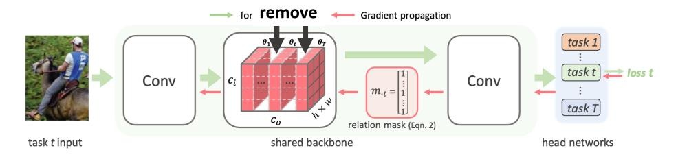
**GradSplit updates parameter**  $\theta_t$  using the gradients from only a subset of tasks  $\{t'\}$ , where the relationship task  $t' \rightarrow t$  is not negative, while discarding gradients from the other tasks.
